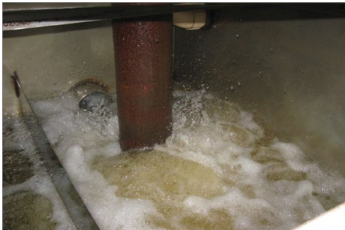
Steel pipe corrosion in highly aerated stainless steel tank
